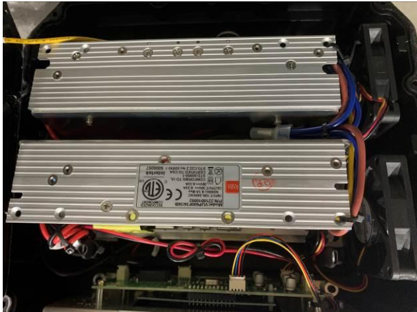
Photo 7 After the dust-proof test, no dust entry into internal.
