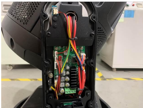
Photo 11 After the waterproof test, no water entry into internal.
