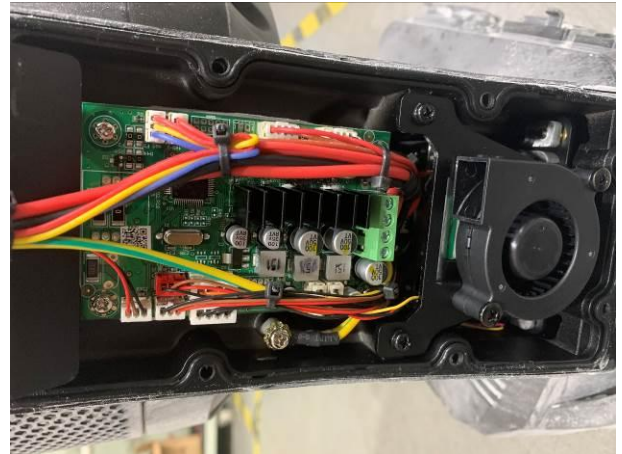
Photo 8 After the dust-proof test, no dust entry into internal.
