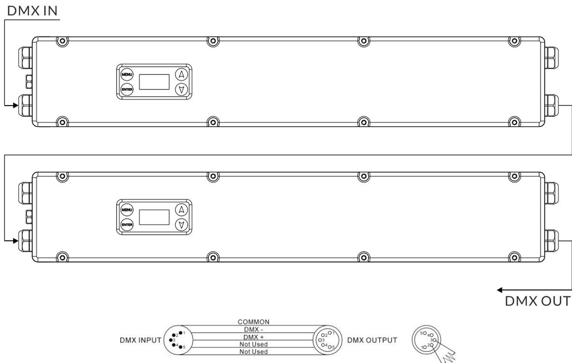
1. At last unit, the DMX cable has to be terminated with a terminator. Solder a 120-ohm 1/4W resistor between pin 2(DMX-) and pin 3(DMX+) into a 3-pin XLR-plug and plug it in the DMX-output of the last unit.
